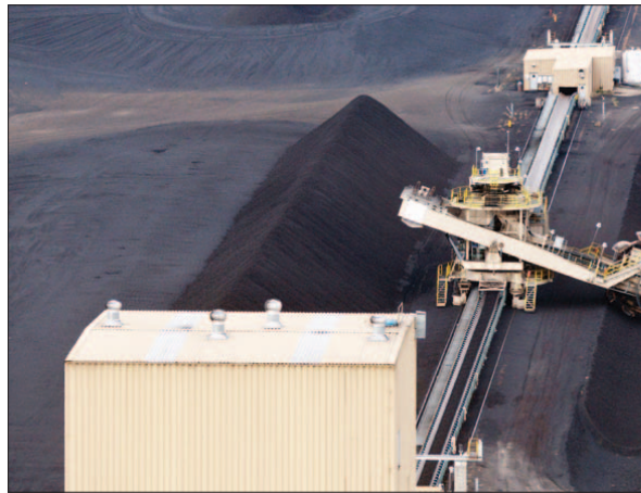
A stacker reclaimer digs up scoops of coal to feed a conveyer belt that feeds the 600-megawatt Boardman Coal Plant.
